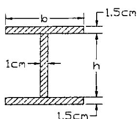
$$F_y = 2400 \text{ kg/cm}^2 \quad E = 2/1 \times 10^7 \text{ kg/cm}^2$$
